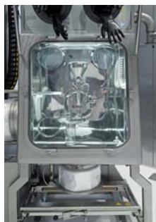
Isolator intergration with active inertisation and oxygen control option
